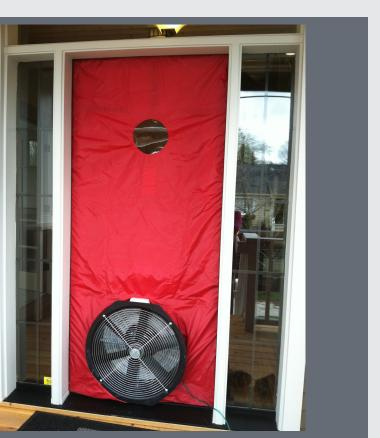
The Front Door is Prepared for a Blower Door test
